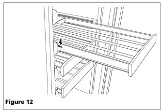
3. Press the left rack release lever (Figure 12) down, and at the same time, lift the corresponding right rack release lever up, and pull the rack out until it is free of the tracks and the cabinet.
