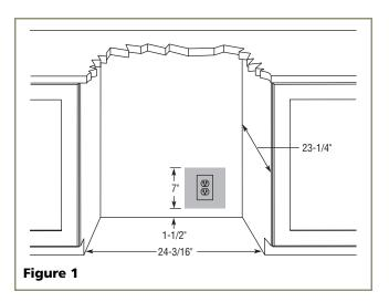
Follow the cut-out drawing in **Figure 1**. The 24-3/16" width allows 1/4" for ease in installation and removal of the unit. 24" is the cabinet depth in most installations. The unit is 23-1/4" deep including the handle on Black and White 2175WC models, 23-1/4" deep including the wood overlay frame on 2175WCOL models and 23-1/4" deep including the door and *not* the handle on Stainless Steel models (see **Figure 2**).
