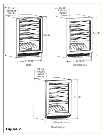
Please note that the unit has adjustable feet that can add one additional inch to height during leveling or to match adjacent cabinets (see **Figure 29** on **Page 13**).
