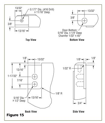
Route notch in top corner of overlay frame as shown (see Top and Side Views). Top of notch is entire depth of frame, front to back.
