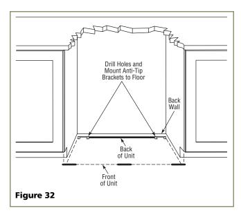
Use a 1/8" drill to make two starter holes and fasten the Anti-Tip Brackets to the floor using the screws provided.
