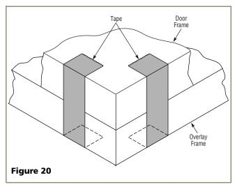
3. Secure the front of the door to the back of the overlay frame using tape on all four corners, as shown in **Figure 20**. Make sure all four edges are aligned.
