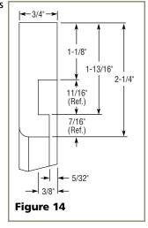
Create a relief for pivot plate by cutting notch in top corner and coinciding back corner of overlay frame.
