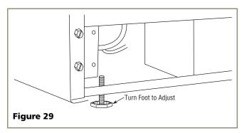
3. Check the levelness after each adjustment and repeat the previous steps until the unit is level. Go on to **8 Install the Unit**.
