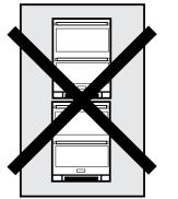
The Anti-tip Bracket must be installed on this unit before it is used. Double stacking units may cause serious personal injury.
