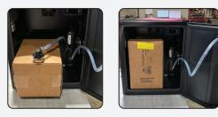
Place the BIB inside the kegerator with easy access to the connection.
