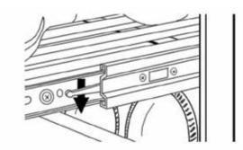
The shelves are removable to help with cleaning and maintenance. To remove a shelf, pull it out as far as you can. There are levers on each side of the shelf near the rollers. Lift the lever on the left hand side and push down the lever on the right hand side to release the shelf from the tracks.
