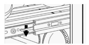
The shelves are removable to help with cleaning and maintenance. To remove a shelf, pull it out as far as you can. There are levers on each side of the shelf near the rollers. Lift the lever on the left hand side and push down on the lever on the right hand side to remove the shelf from the tracks.
